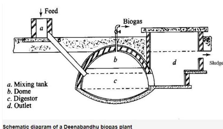
Biogas is a mixture of methane and carbon dioxide. It also has traces of hydrogen sulphide (3%), ammonia, oxygen, hydrogen, water vapour etc., depending upon feed materials and other conditions. Biogas is generated by fermentation of cellulose rich organic matter under anaerobic conditions. In anaerobic conditions, the methane-producing bacteria become more active. Thus, the gas produced becomes rich in methane. The optimum utilization depends upon the successful
