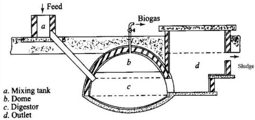
Schematic diagram of a Deenabandhu biogas plant
